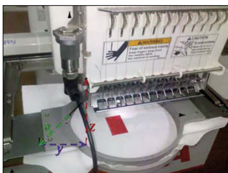
Fig. 4. The HAPPY embroidery machine with the sensor installed vertically
